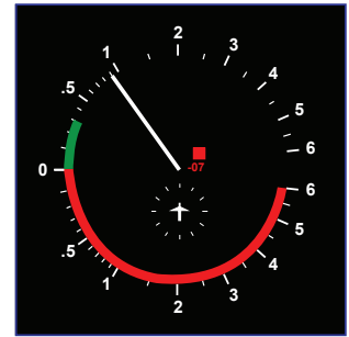
Fig 9: A weakening "level off" RA as shown on a generic IVSI display
